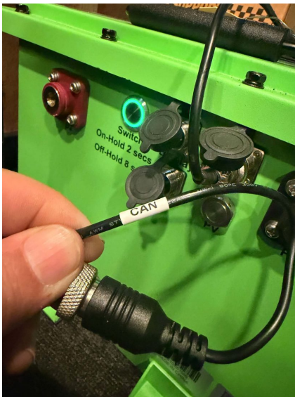
CAN lead to CAN port
